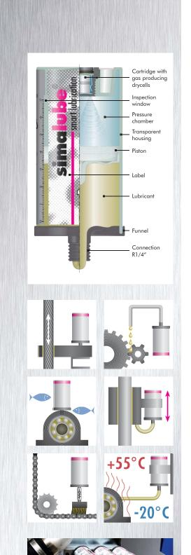
The globally patented simulube® lubricant dispensers reliably provide the individual lubrication points with the required amount of lubricant - 24 hours a day. The dispensers are continuously adjustable for periods of between 1 and 12 months.
